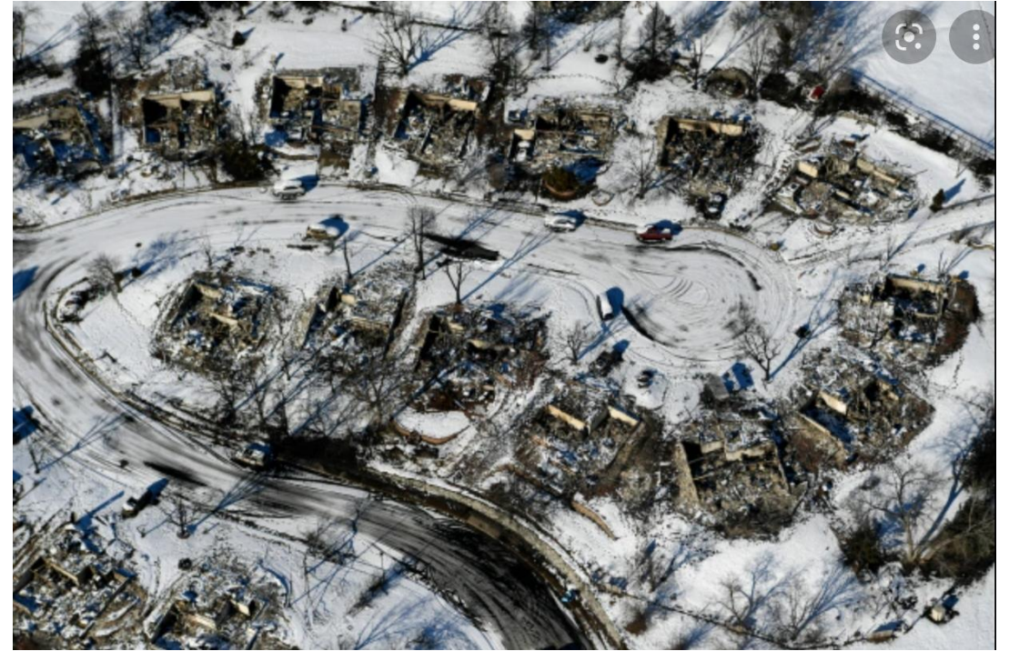
Neighborhood in Superior destroyed by embers and radiant heat.
